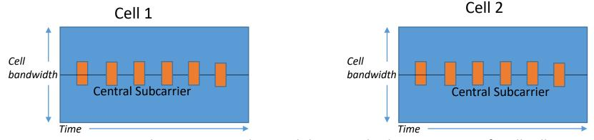
4G – Sync signals are positioned around the central subcarrier – same for all cells. Leads to interference between cells.
